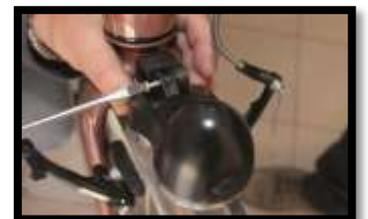
12. Place the pedals according to the sides. Screw the pedals using wrench number 15. Remember that pedals must be threaded clockwise to avoid that unscrews during your ride.
