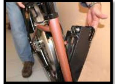
6. Take off the plastic protector from the handlebar. Switch the handlebar to the front and screw using allen wrench number 5 and 6 accordingly.
