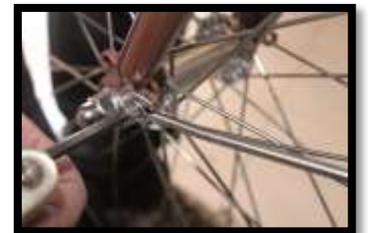
10. Fix the spokes into the front mudguard suport using allen key wrench 6.
