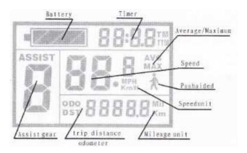
**ASSIST** (Assistance): level of assistance, power of the motor **BATERIA**: remaining battery capacity before recharge
